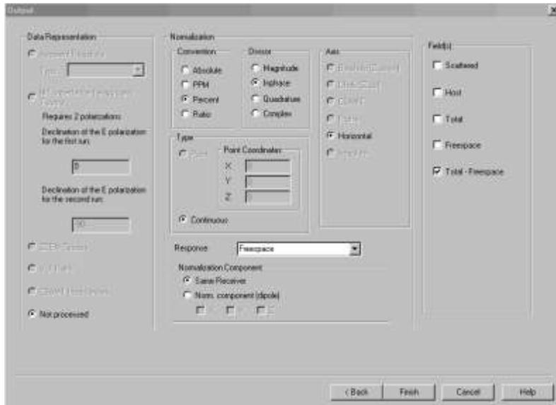
In the example above is the selections for a standard dipole-dipole moving array. Here the data is to be normalized to the Inphase of the primary field and computed in units of Percent. The output fields are Total-FreeSpace and the normalization is Continuous (at each data point) and to the freespace of the same component as the data.
