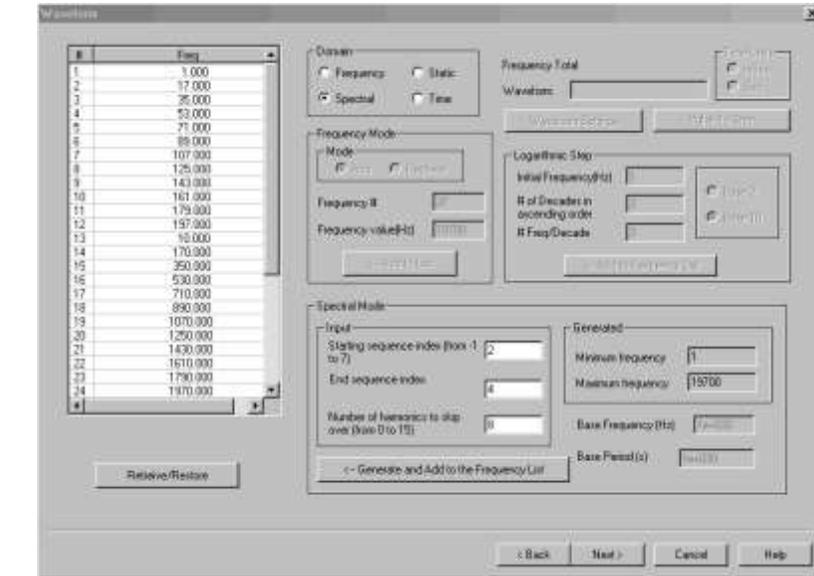
Here you will select whether you wish to calculate a Frequency Domain model, a static (DC) model or a Time Domain survey.
