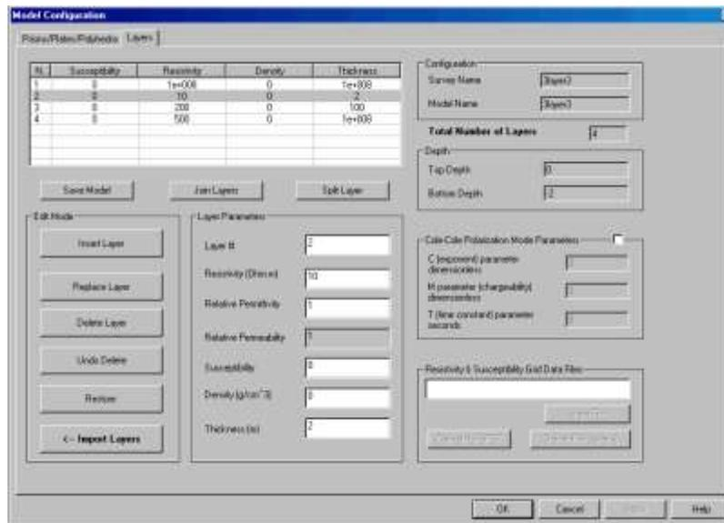
Layers can be defined for the resistivity, thickness, electrical permittivity, magnetic susceptibility and density. Also, the layers can be made polarizable through setting Cole-Cole parameters which is applicable for all EM modeling. The top layer is an air layer by default but can be set with suitable parameters for other applications such as marine or underground. For example, for surveys on the seabed one might set the top layer to be the conductivity of sea water.
