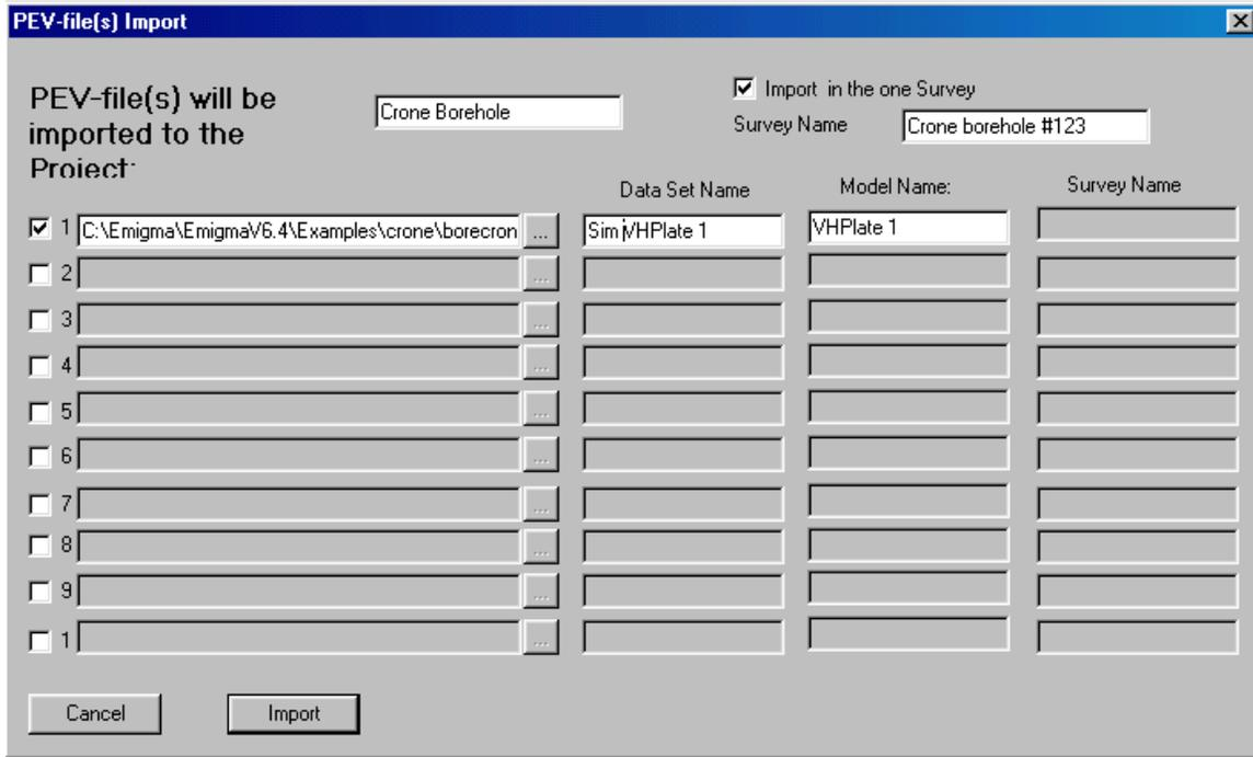
Browse for the .pev file you would like to import into the database. Select the next checkbox and click the ... button to browse for more .pev files. Repeat the process to import up to 10 pev files at a time.
