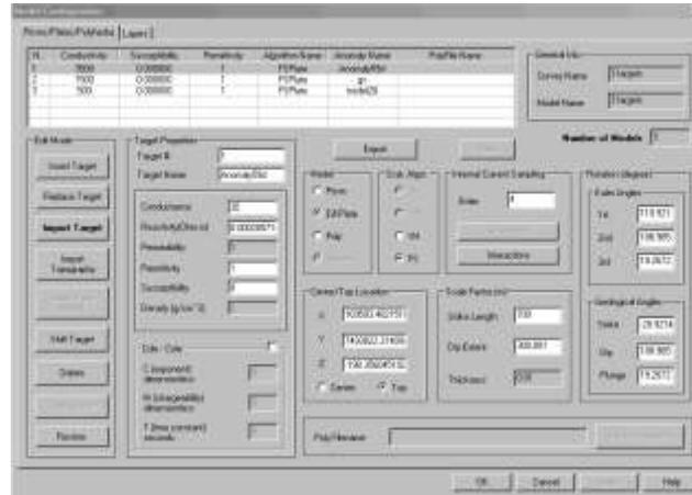
The other tab in Modelgui is for the insertion/editing/deletion of 3D anomalies.
