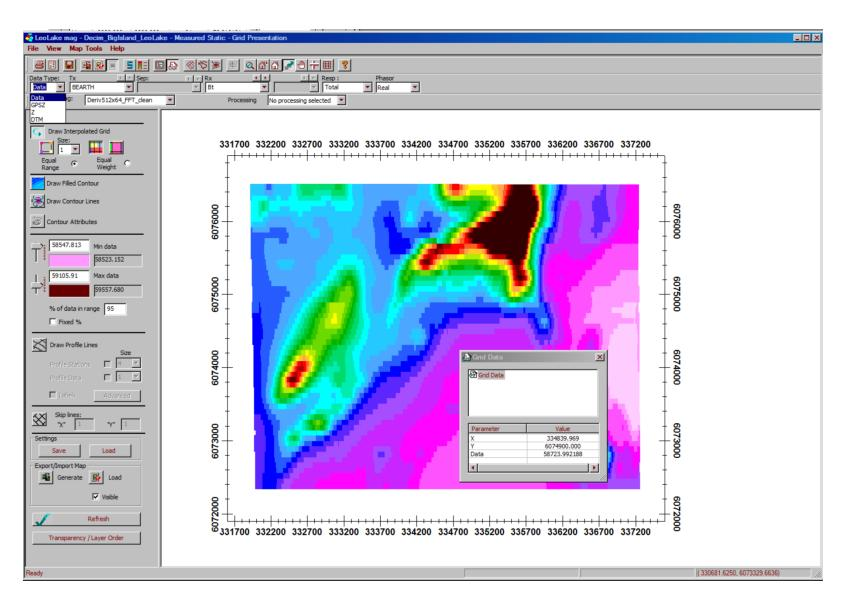
This grid contains Btotal, dB/dx, dB/dy, dB/dz , GPSZ and altimeter data(Z) and calculated Digital Terrain Model. Initially, grid is not interpolated
