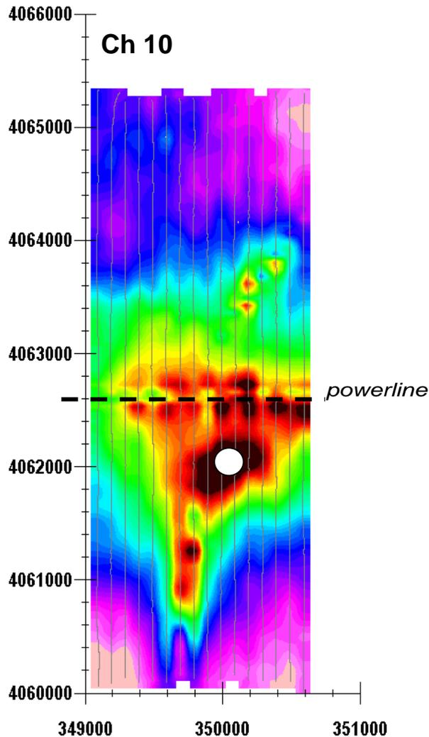
\*The white circle marks the approximate center of the pipe, based on drill hole results.
