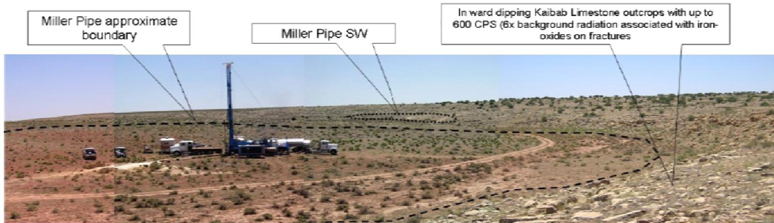
Red Moenkopi mudstone down-dropped into shallow surface depression of inward dipping Kaibab limestone – Miller Pipe; Drilling in progress on VANE drill hole #691-2; view looking southwest
