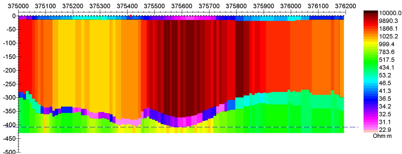
For the previous inversions, the data in channels 1-24 were inverted. Channels 25-28 were not used due to the noise in the data. Channels 1-2 were included because they appeared consistent with the rest of the data channels on these lines (see decays on pages 22 and 23 – layered earth models match the first two channels) although these channels do have some quality issues (page 25) across the survey area.
