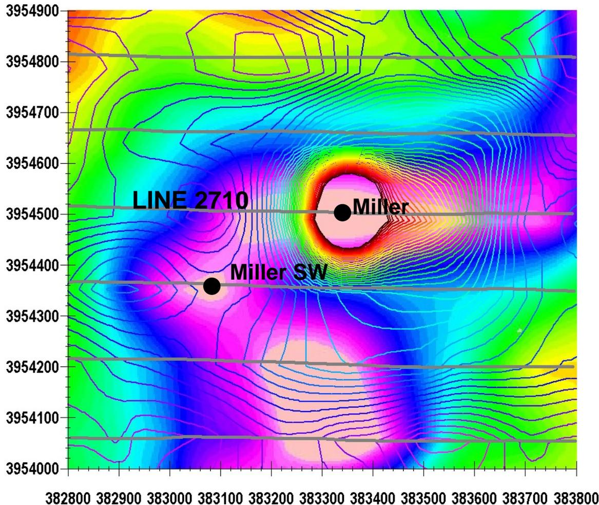
Comparison of the first channel of the EM data (contour lines) with the digital terrain model. Survey lines are also shown.
