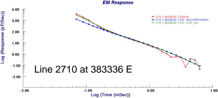
On the left: comparison of the measured data to the background model and prism model for three different time channels along Line 2710. The model fits the general shape of the anomaly. The response of the model is slightly too small for the first three channels.
