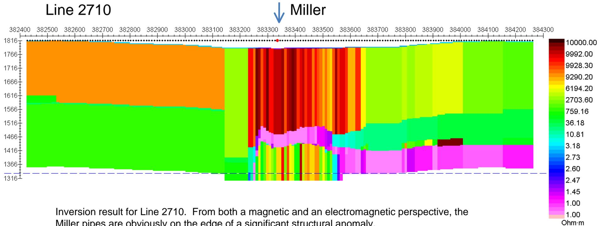
Note: While the inversion clearly shows a structural anomaly in the vicinity of Miller, the anomaly appears to be significantly 3D in nature and the stacked 1D inversion approach is not considered to be sufficiently accurate. This is analogous to the response at FTSE.
