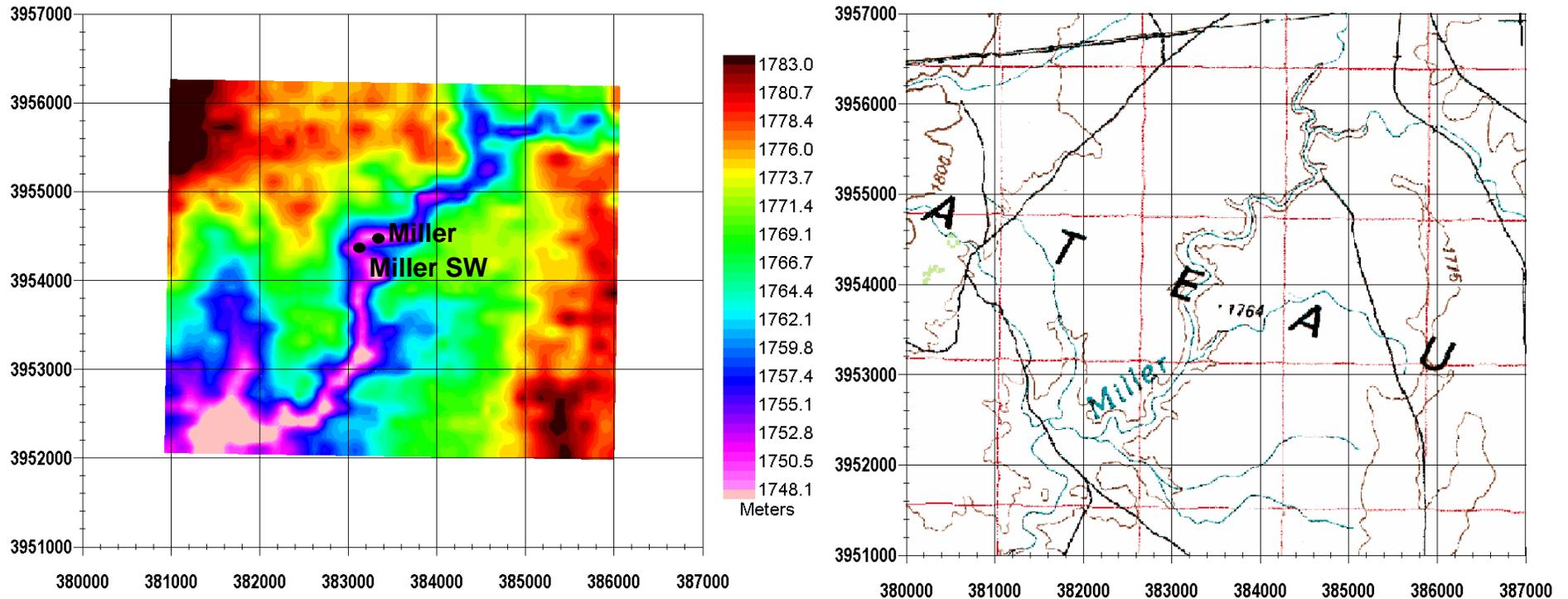
The digital terrain model on the left was calculated from the altitude and GPS Z channels in the VTEM data. Both of these pipes appear to be in a small canyon, with an elevation about 15 m below that of the surroundings. According to Google Maps, this is the Miller Wash.
