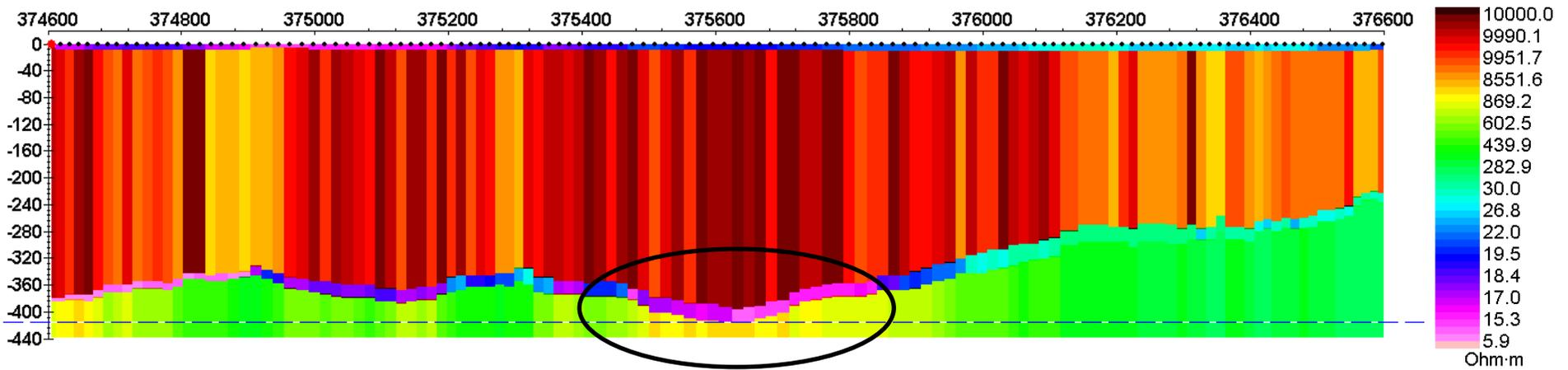
Above is a stacked 1D inversion over Line 3750, which is about 60 m south of the pipe. (A slightly longer section of the line was inverted than on 3720). Note the thinning of the resistive layer to the east.
