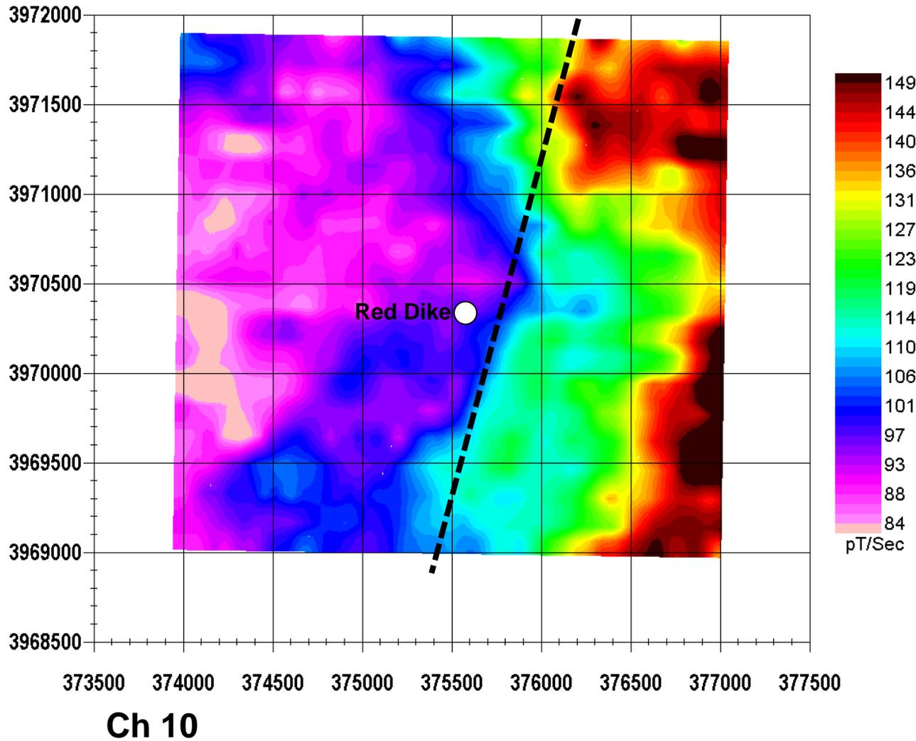
Map of the mid time (channel 10) data over a 3 km x 3km area around Red Dike. The linear high that was visible at early times (position marked by dashed line) is not seen here; however, to the west of the early-time anomaly, the response is much lower than to the east.
