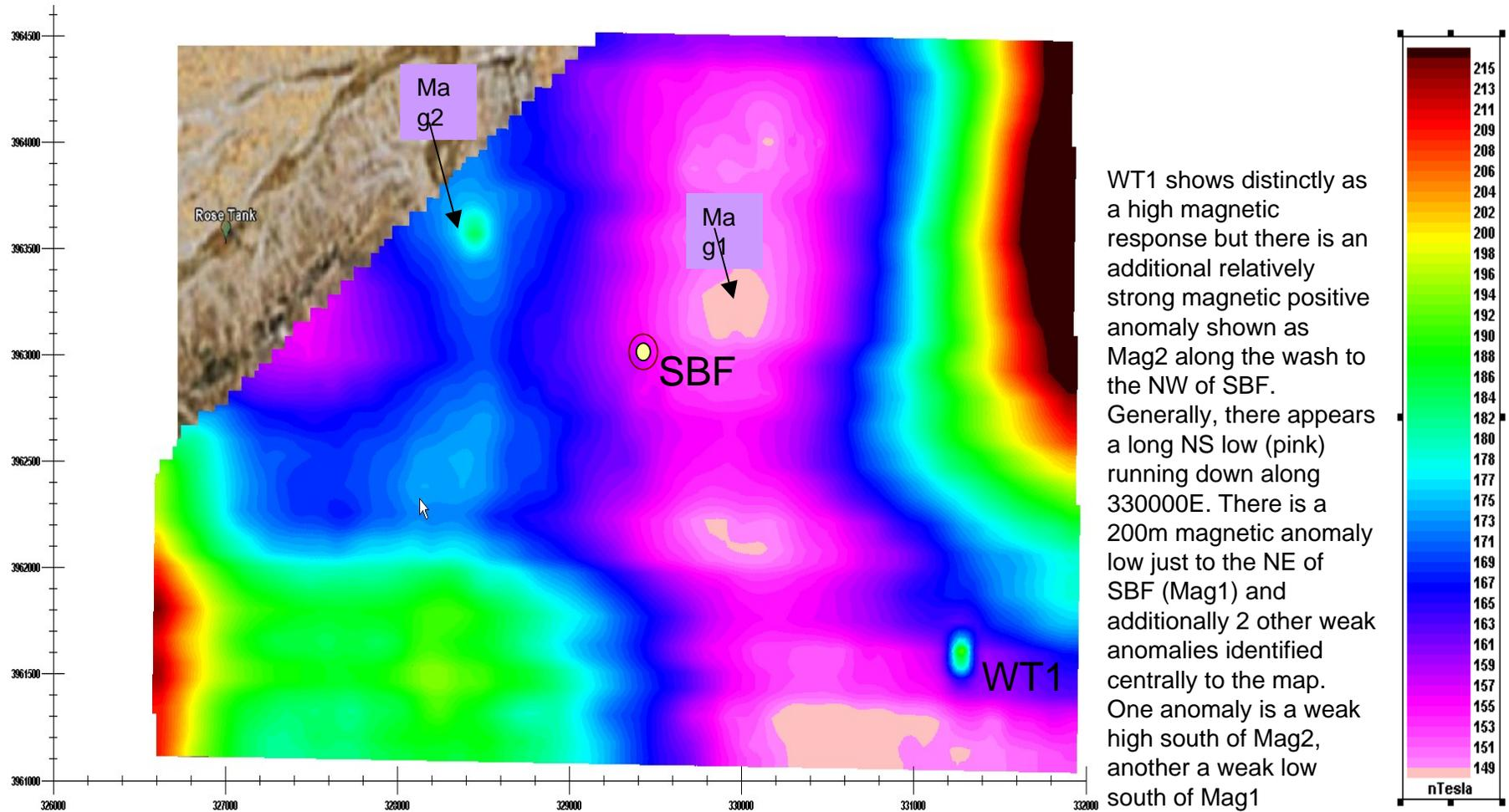
WT1 shows distinctly as a high magnetic response but there is an additional relatively strong magnetic positive anomaly shown as Mag2 along the wash to the NW of SBF. Generally, there appears a long NS low (pink) running down along 330000E. There is a 200m magnetic anomaly low just to the NE of SBF (Mag1) and additionally 2 other weak anomalies identified centrally to the map. One anomaly is a weak high south of Mag2, another a weak low south of Mag1
