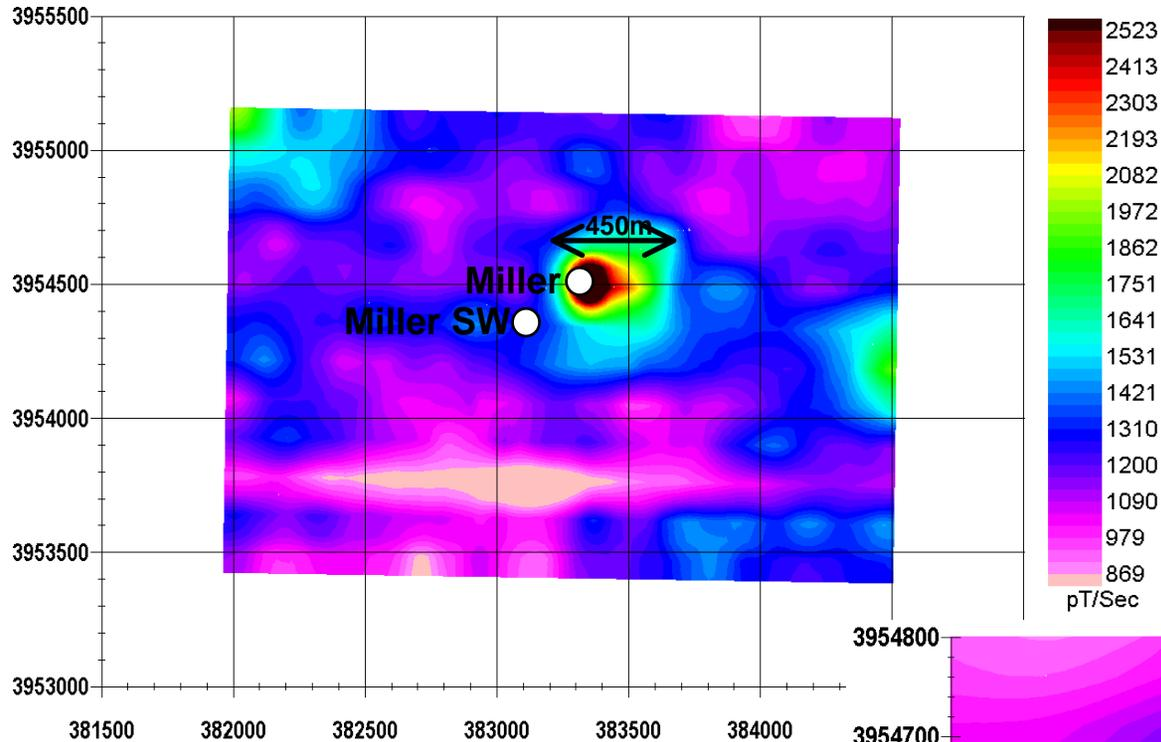
Above: The first channel of the EM data over the same area as the magnetic data shown on the previous page. There is a strong anomaly in the vicinity of the Miller pipe covering a relatively large area.
