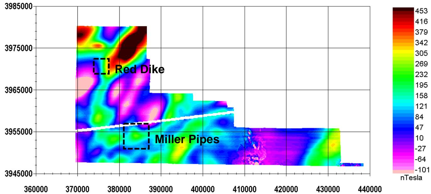
Magnetic field with background (IGRF) response removed over the NE section of the VTEM survey. Red Dike is on the edge of a large magnetic high.
