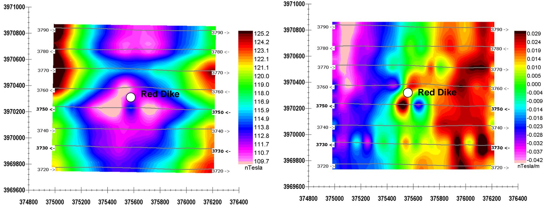
Left: Close up of the magnetic response around Red Dike with the gradient removed. In this contour plot, there is an anomalous high just south of Red Dike. \*\*While this anomaly appears south of Red Dike, Red Dike is half-way between Lines 3750 and 3760, which are 150 m apart. Due to this line spacing, there is limited resolution of the response north-south.
