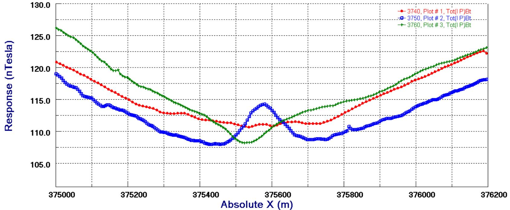
Plot of the magnetic data (gradient removed) along Lines 3740-3760. Red Dike is in between 3750 and 3760.
