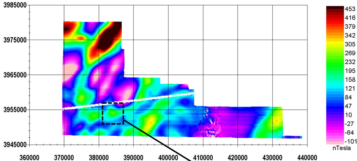
Above: Magnetic field with background response removed over the NE section of the VTEM survey.
