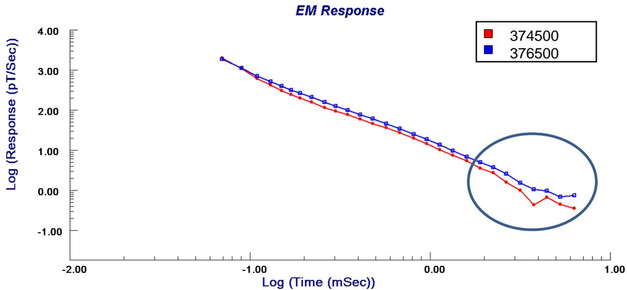
The plot shows two decays along Line 3750, the first at 374500 (red), which is west of the linear anomaly, and the 2 km east at 376500 (blue), which is east of the linear anomaly. Note the difference between them – the decay at 376500 has a greater amplitude across all but the earliest time channels. This suggests a difference in structure at depth.
