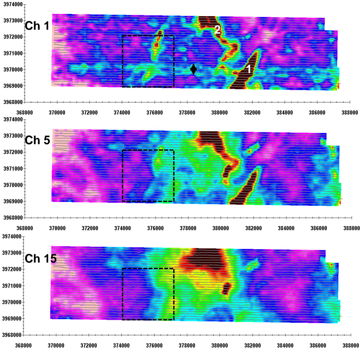
EM response at three different channels over a larger (18 km x 4 km area). At early channels, there are other linear anomalies to the east, one trending at a similar azimuth to the anomaly near red dike. Another linear anomaly (2), trends approximately northwest.
