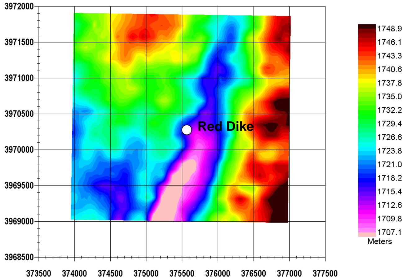
The digital terrain model was calculated from the altitude and GPS Z channels in the VTEM data. Red Dike is on the edge of a low in the topography.
