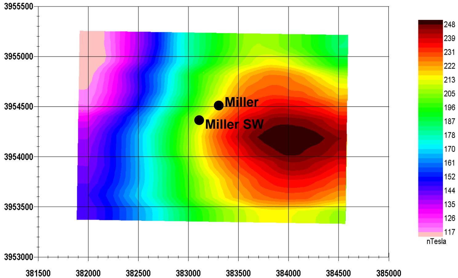
Close-up of magnetic response (2.5 km x 2km area) near the Miller pipes. These pipes are on the edge of a magnetic anomaly much like all of the known pipes on the North Rim.
