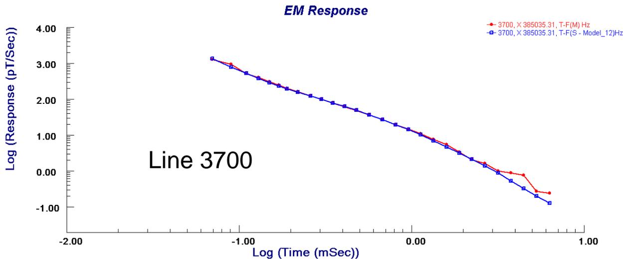
Because of the issues with the early time data on certain lines, as seen on the previous page, as well as some difficulty with matching early-time data in modeling, the response was studied more carefully on a series of lines at an easting where there are no significant anomalies.
