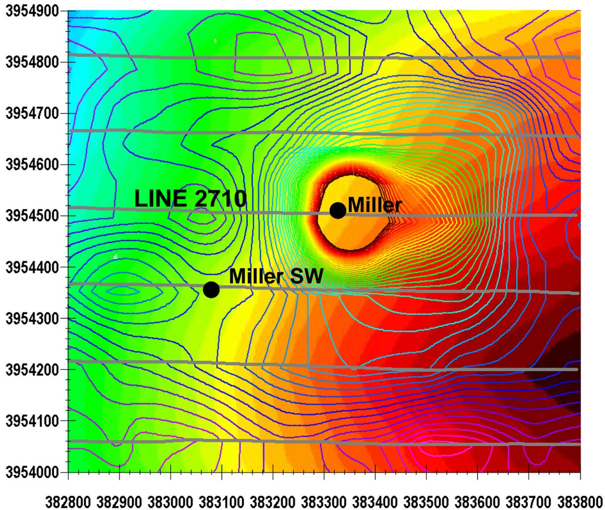
Comparison of the first channel of the EM data (contour lines) with the magnetic field. Survey lines are also shown.
