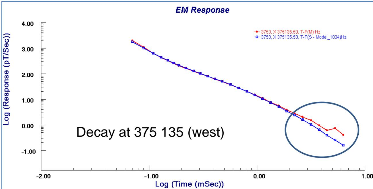
The top plot shows the fit of the west background model to the measured data at a point west of Red Dike. The bottom plot shows the fit of the east background model to the measured data at a point east of Red Dike.
