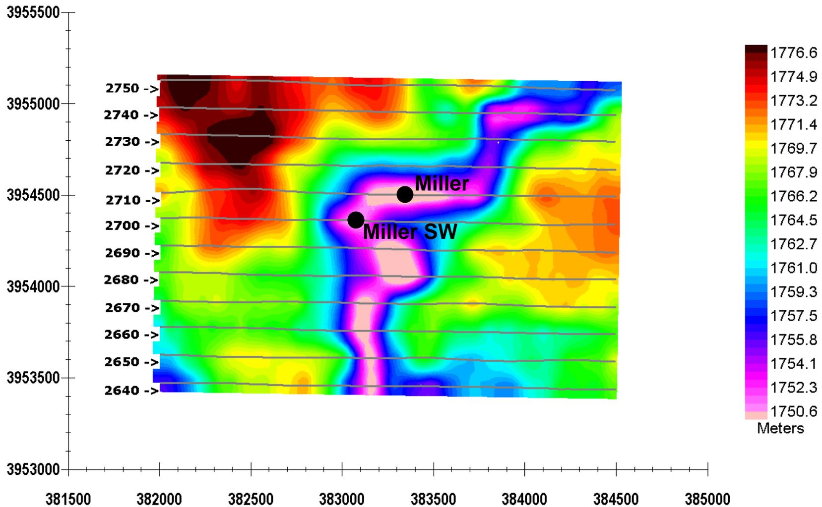
Close-up image of the digital terrain model, with the pipe locations marked.
