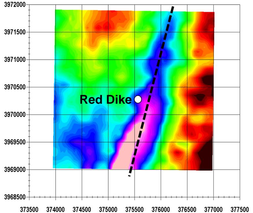
Comparison of the EM data with the digital terrain model. There is a clear correlation between the linear high in the EM data at early times and the area of low topography (a wash).
