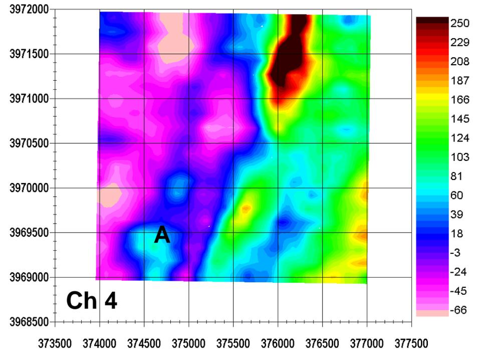
Maps of the data in which the response of the West Background model has been removed (this removes effects due to altitude variation of the plane). The data on lines 3720-3750 has been shifted so that Channel 1 matches the rest of the data (as on page 24).
