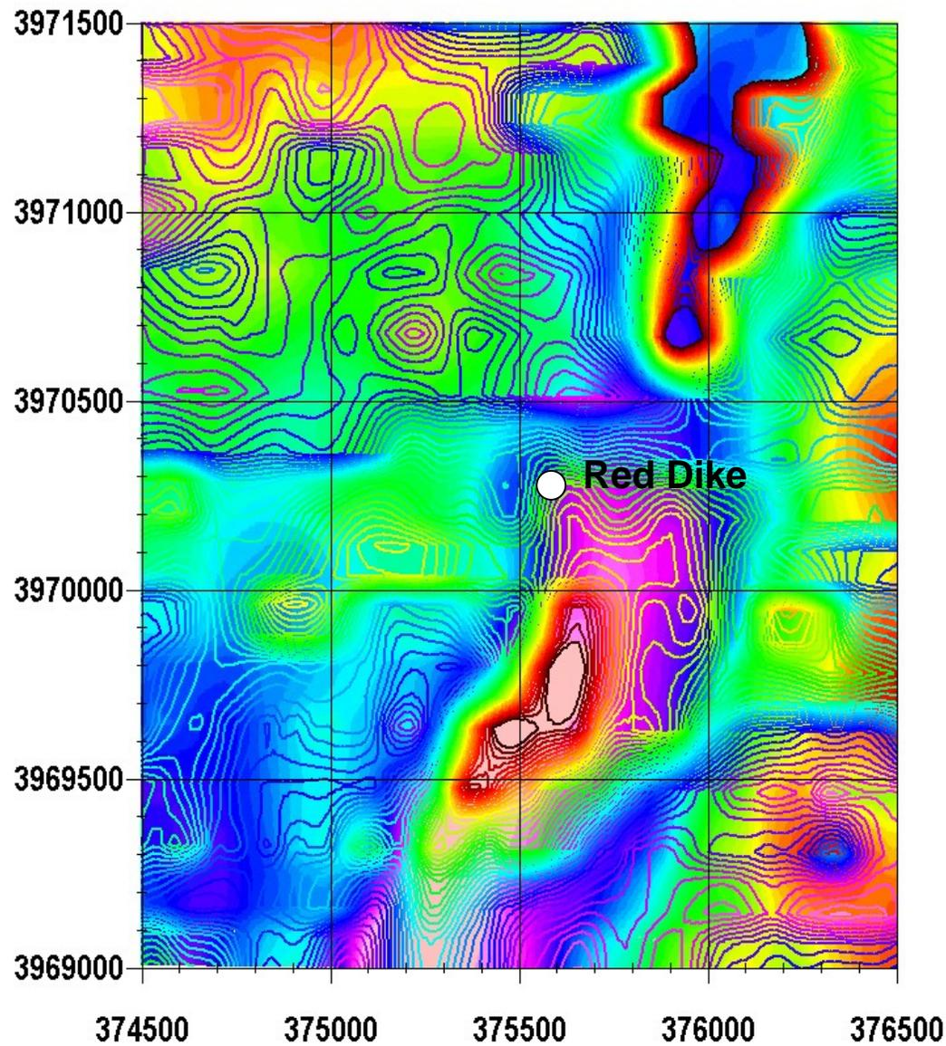
Close-up comparison of the first channel of the EM data (contour lines) with the digital terrain model.
