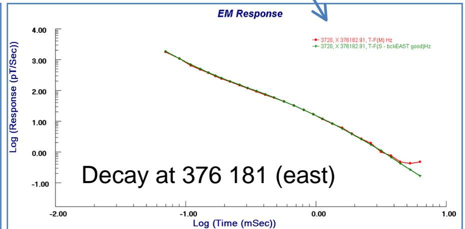
These two background models fit the data along Line 3720 well. Unlike on Line 3750 (previous page), they fit the late-time response of the data, although the last 4-6 channels are noisy.
