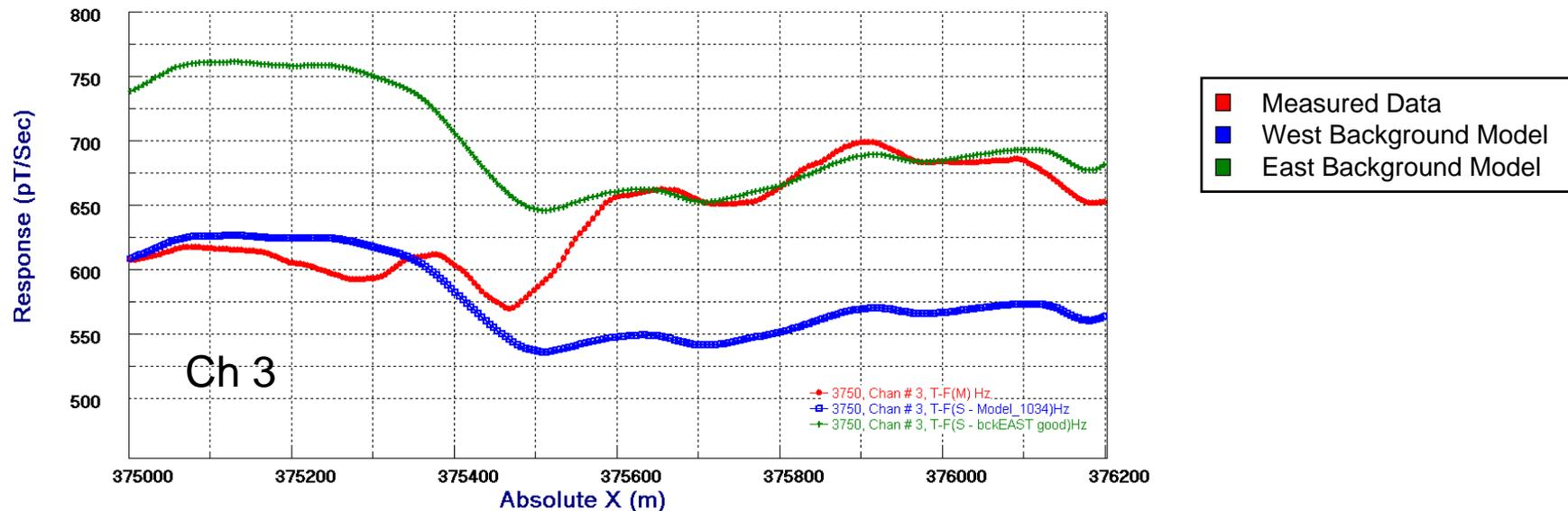
Two models were needed to fit the background EM response near Red Dike. One model fits the data to the west of the anomaly, and the other fits the data to the east of the anomaly. In both of these models, resistivity varies only with depth. The two models have the same four layers, but the model for the east section has a thinner resistive layer (270 m vs. 310 m) and a slightly thicker overburden. This increases the EM response.
