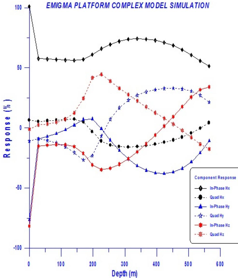
The data plotted in the figure above are the total measured field minus the free space field in all three borehole components at 30Hz. The data have been continuously normalized as a percentage to the total magnetic field at the RX station. HZ is the axial borehole component pointing up the hole, HX is horizontal and perpendicular to the borehole while HY is defined according to a right handed system such that z is positive up along the borehole.
