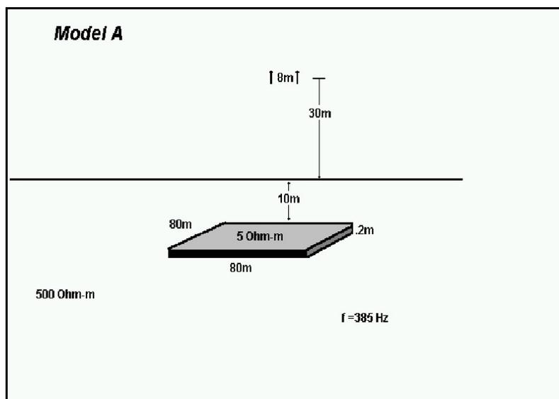
in a 500 Ohm-m halfspace. A coplanar system is being towed 30m above the ground with a 8m separation and is operating at 385Hz. We show the response from the center of the plate out to 160 metres from its center.
