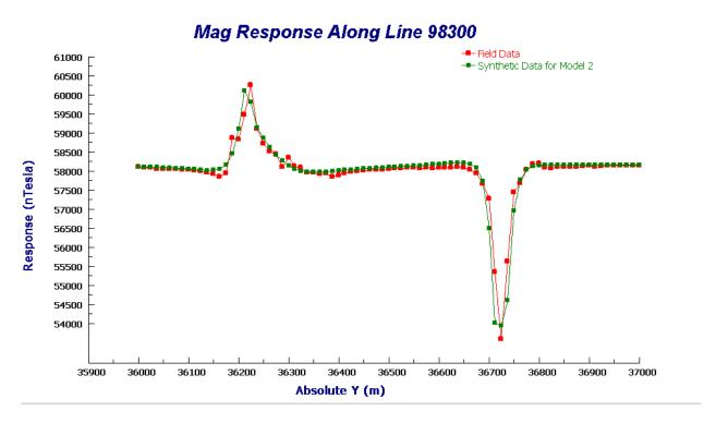
Figure 12b: Comparison of the magnetic response along Line 98300 for the field data and the synthetic data from Model 2.
