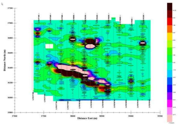
Figure 6: A plot of the derivatives of the magnetic field in the north-south direction. Points that were extrapolated outside a radius of 50 m have been removed.
