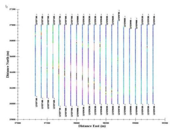
Figure 1: The profile lines for the magnetic survey, showing the data.
