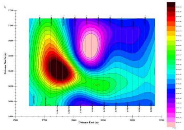
Figure 7: A contour fill of the data after interpolation and upward continuation to a height of 300 m.
