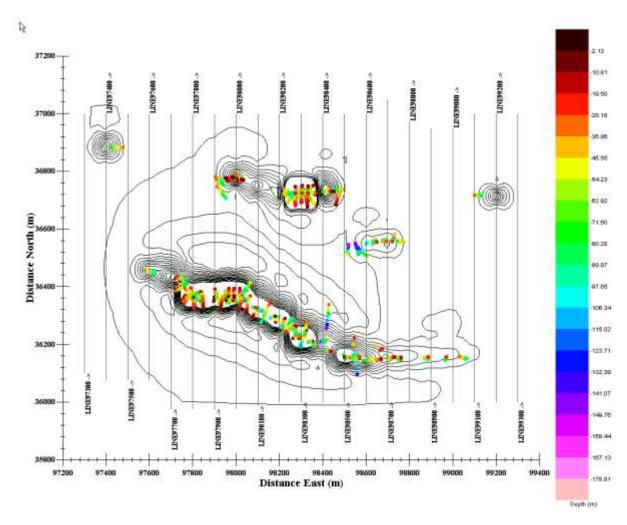
Figure 10: A contour plot of the synthetic data showing the Euler solutions following a deviation error removal of 15%, and an uncorrelated solution removal of 35% with a minimum cluster size of 10 m. A window of 50 rows by 8 columns, a transverse moving step of 12 rows, and an inline moving step of 2 columns were used.
