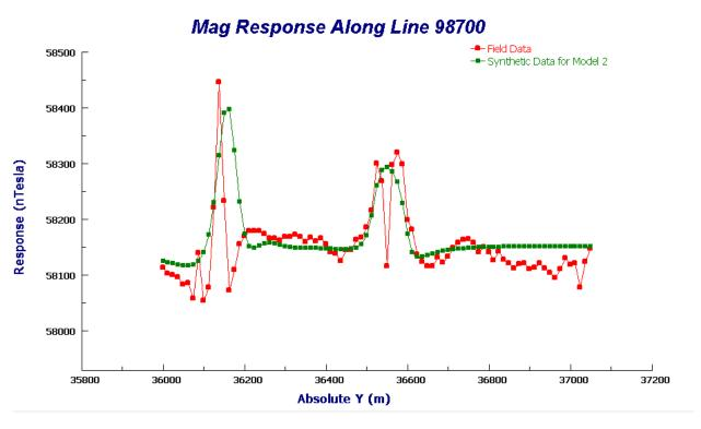
Figure 12c: Comparison of the magnetic response along Line 98700 for the field data and the synthetic data from Model 2.
