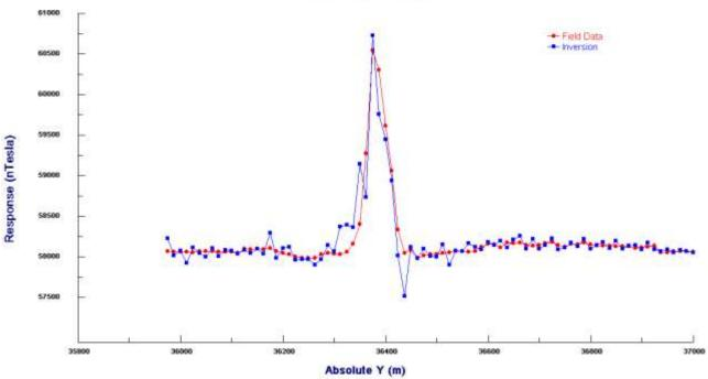
Figure 17a: Comparison of the magnetic response along Line 97 800 for the field data and the synthetic data for the model from the inversion in Figure 15.
