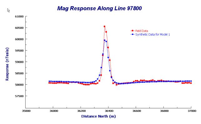
Figure 5a: Comparison of the magnetic response along Line 97800 for the field data and the synthetic data from Model 1.
