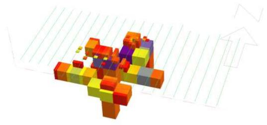
Figure 15c: The model resulting from a fine optimization inversion of the field data, using Model 2 as a starting point. Cells with susceptibilities less than -0.02 are shown.
