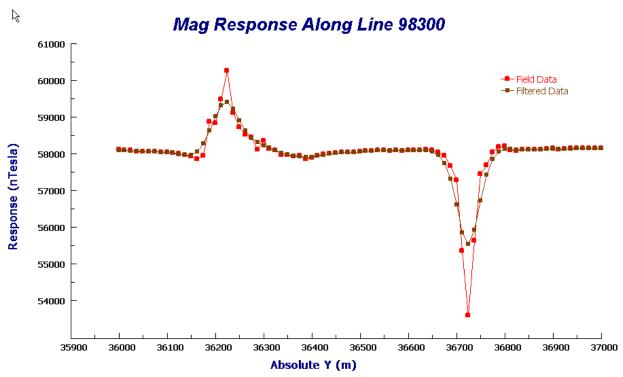
Figure 13: Comparison of the magnetic response along Line 98300 for the field data and the data after 1-D Gaussian filtering. A radius of 74.762 m and a deviation of 18 m were used.
