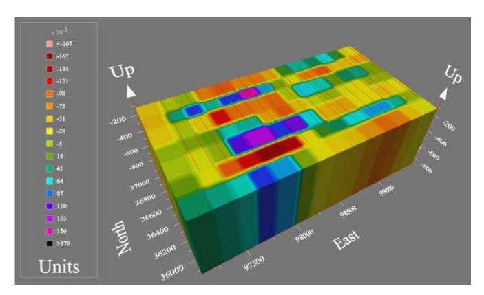
Figure 14: A 3-D contour of the data resulting from a matrix inversion of the field data. The depth of the surface shown is 120 m.
