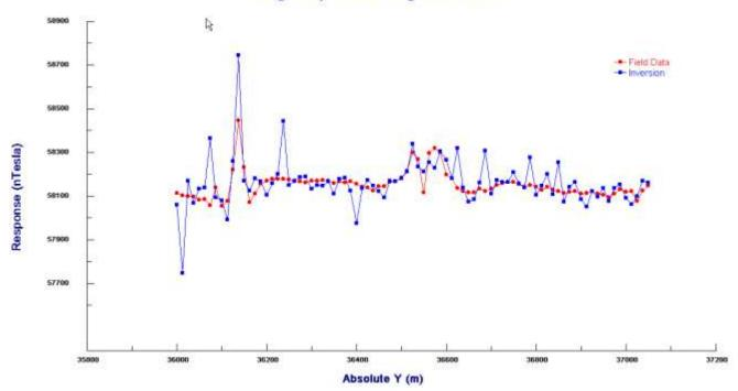
Figure 17c: Comparison of the magnetic response along Line 98700 for the field data and the synthetic data for the model from the inversion in Figure 15.
