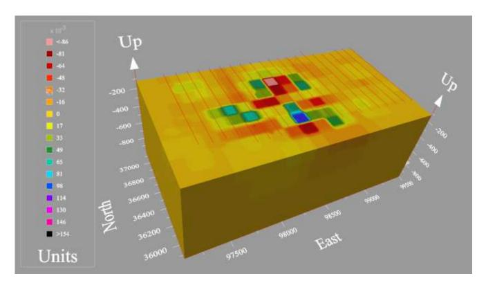
Figure 16: A 3-D contour of the data for Model 15. The depth of the surface shown is 120 m.
