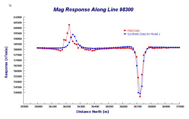
Figure 5b: Comparison of the magnetic response along Line 98300 for the field data and the synthetic data from Model 1.
