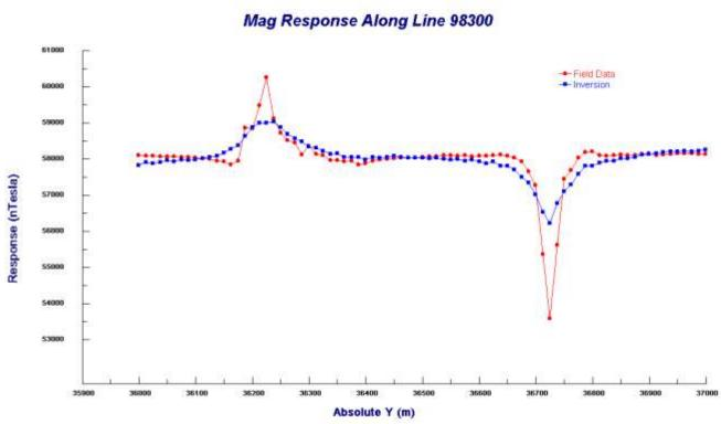
Figure 17b: Comparison of the magnetic response along Line 98300 for the field data and the synthetic data for the model from the inversion in Figure 15.
