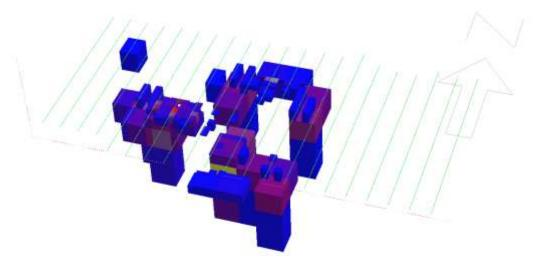
Figure 15b: The model resulting from a fine optimization inversion of the field data, using Model 2 as a starting point. Cells with susceptibilities greater than 0.02 are shown.
