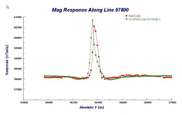
Figure 12a: Comparison of the magnetic response along Line 97800 for the field data and the synthetic data from Model 2.
