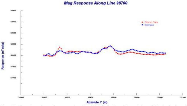
Figure 18: Comparison of magnetic response along Line 98700 for the filtered data and the synthetic data for the model from the inversion of the filtered data.
