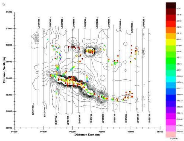
Figure 8: A contour plot of the interpolated data showing the Euler solutions following a deviation error removal of 15%, and an uncorrelated solution removal of 35% with a minimum cluster size of 10 m. A window of 50 rows by 8 columns, a transverse moving step of 12 rows, and an inline moving step of 2 columns were used.
