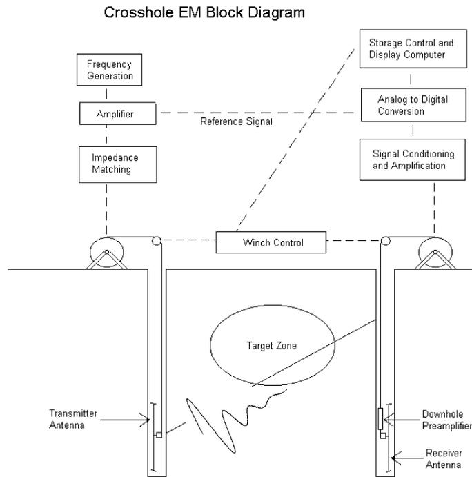
**components and standard survey setup.**
