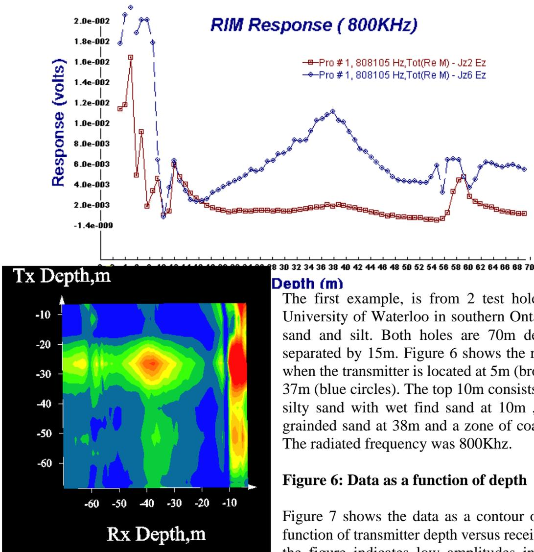
The first example, is from 2 test holes located at the University of Waterloo in southern Ontario in an area of sand and silt. Both holes are 70m deep, vertical and separated by 15m. Figure 6 shows the received response when the transmitter is located at 5m (brown squares ) and 37m (blue circles). The top 10m consists of fine sand and silty sand with wet fine sand at 10m , muddy medium grained sand at 38m and a zone of coarse sand at 57m. The radiated frequency was 800Khz.
