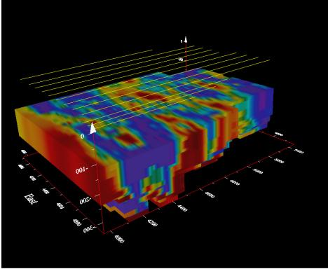
3D Resistivity Inversion Sliced at 100m depth
